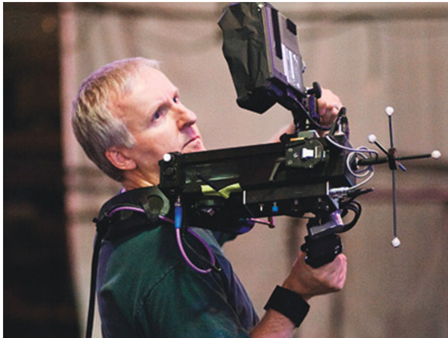
Figure 2.5: James Cameron uses one of the virtual camera control rigs on the set of Avatar . [34]
