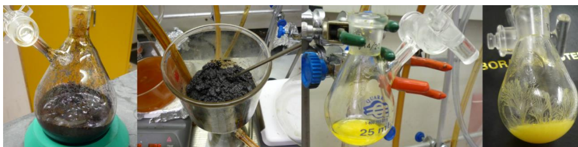
Figure 2-8. From left to right: Skraup reaction mixture before work-up; side product, acrolein polymer; 8-bromo-6-methylquinoline after distillation; solidified 8-bromo-6-methylquinoline.
