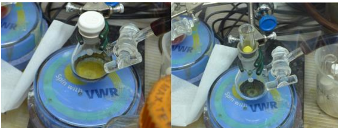
Figure 3-6. Left: Removal of all volatiles before filtration. Right: Filtration through a fritted funnel.
