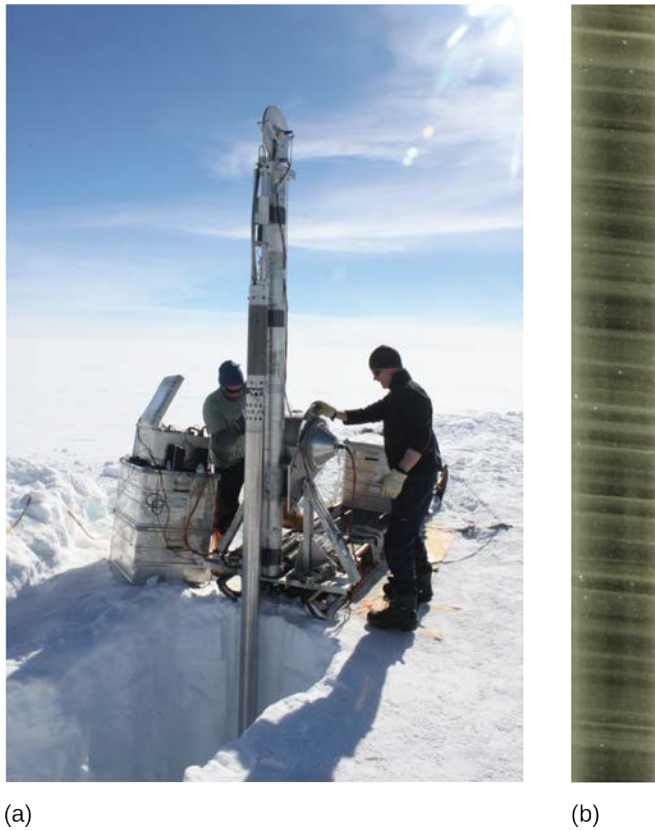
Figure 44.26 Scientists drill for ice cores in polar regions. The ice contains air bubbles and biological substances that provide important information for researchers. (credit: a: Helle Astrid Kjær; b: National Ice Core Laboratory, USGS)
