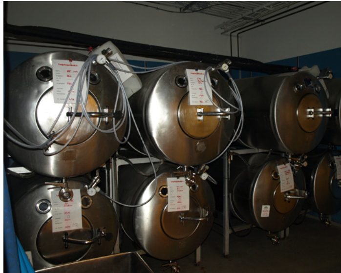
Figure 7.15 Fermentation of grape juice into wine produces CO 2 as a byproduct. Fermentation tanks have valves so that the pressure inside the tanks created by the carbon dioxide produced can be released.
