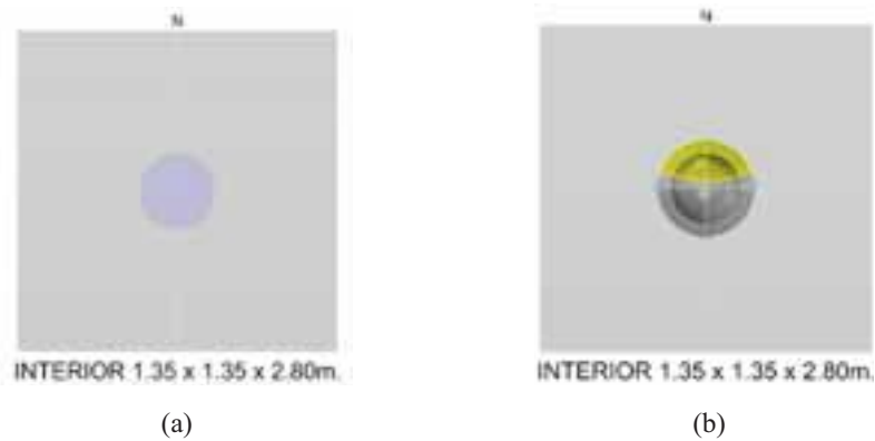
Fig. 3: Simulation model: One unit (a) Base case (Circular translucent material, \tau = 60\% ) (b) Original SDV & Modified SDVs ( \tau = 40\% , 50\% , and 60\% )
