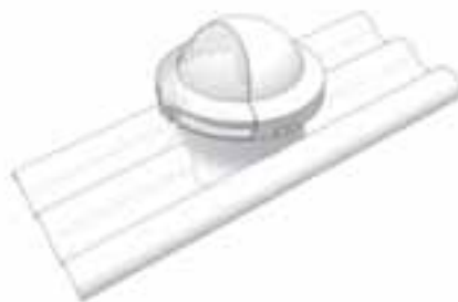
Fig. 1: An integrated skylight and shading dome with natural ventilation (SDV)
