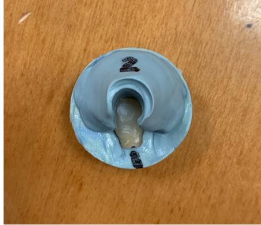
Figure 4. Vinyl polysiloxane molds (A) for accurate repeated positioning for spectrophotometer readings (B)
