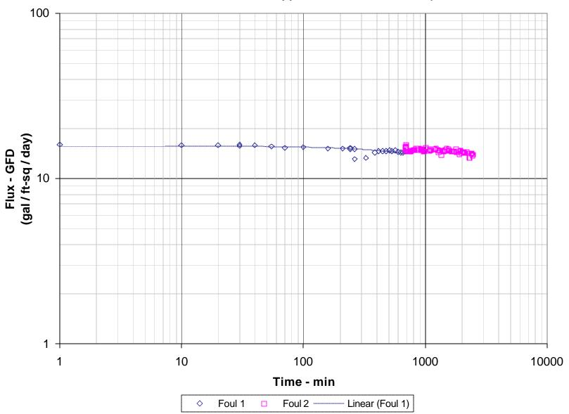
Standard Fouling Test for the Selected Membrane J - Flux vs. Time (Selected Operating Pressure = 550 psi and Operating Flow Rate = 10 gpm, 12500 ppm TDS Produced Water)
