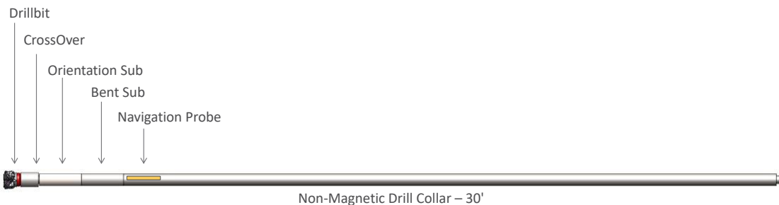
Figure 2.15: Bottom hole assembly configuration used in the development of the drilling simulator.
