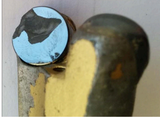
Figure 4.2: Severe bit whirl caused bit damage that would in turn reduce ROP for the duration of the drilling interval, and increase the risk of pipe failure, after [2].
