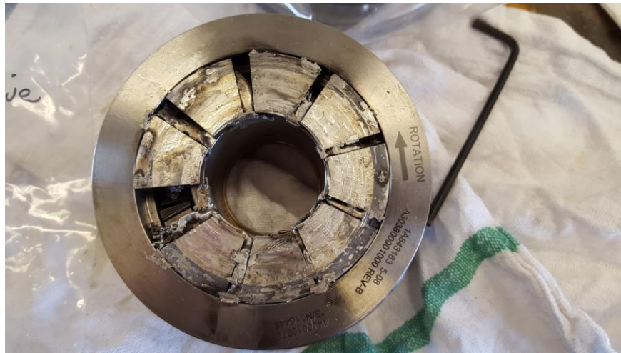
Figure 15: Pinion 2 Inactive Thrust Bearing Damage
