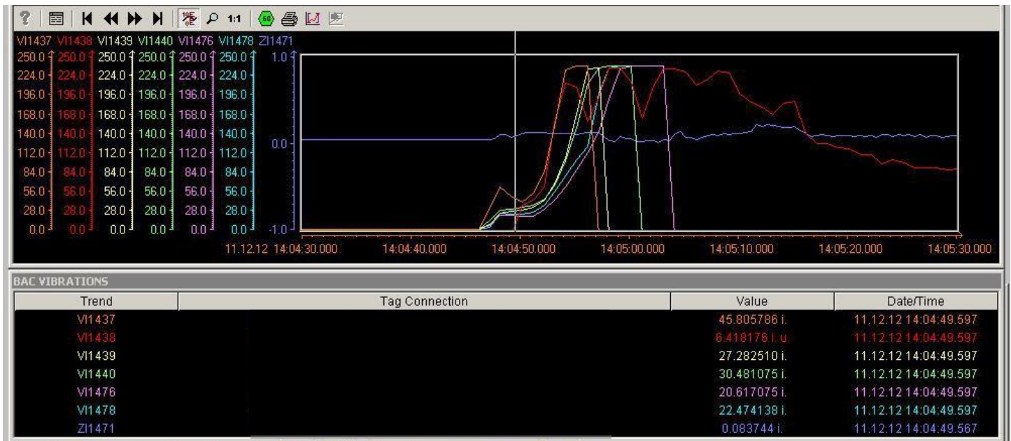
Figure 5: Start-Up Vibration Trends During Failure
