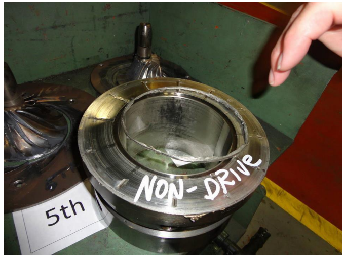
Figure 8: Normally Unloaded Bullgear Thrust Bearing
