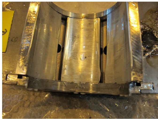
Figure 3: Damaged Pinion Bearing
