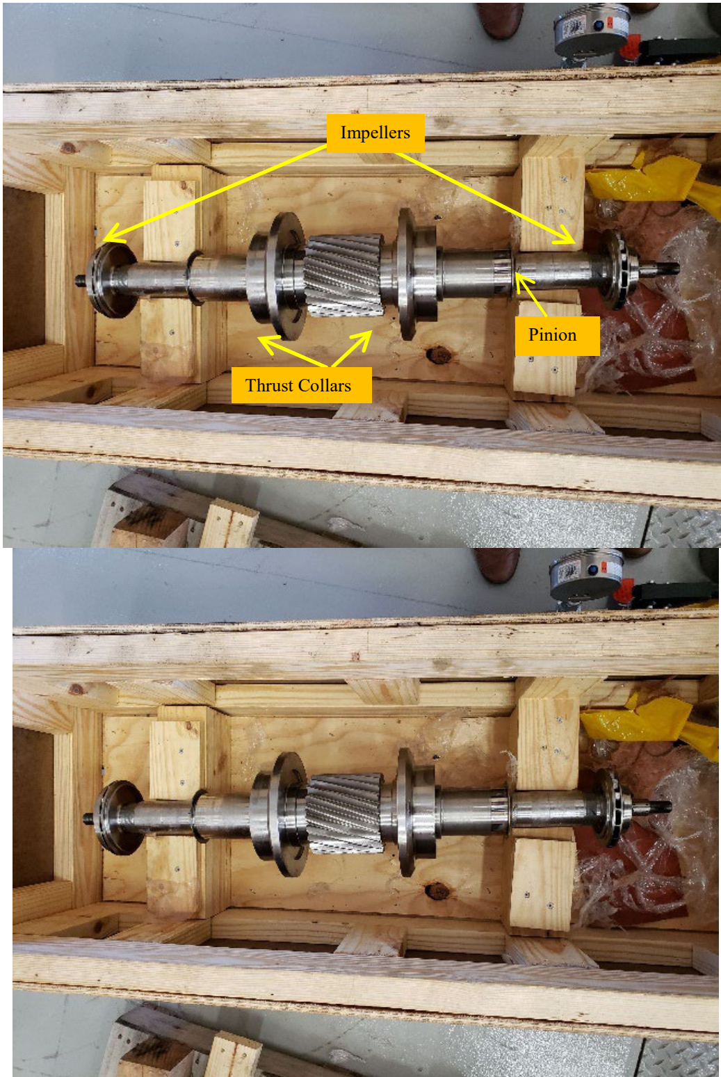
Figure 19. Compressor Pinion shaft with Thrust Collars and Impellers Mounted
