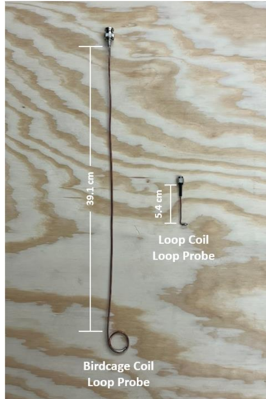
Figure 5: Loop Probes for the Birdcage and Loop Coils
