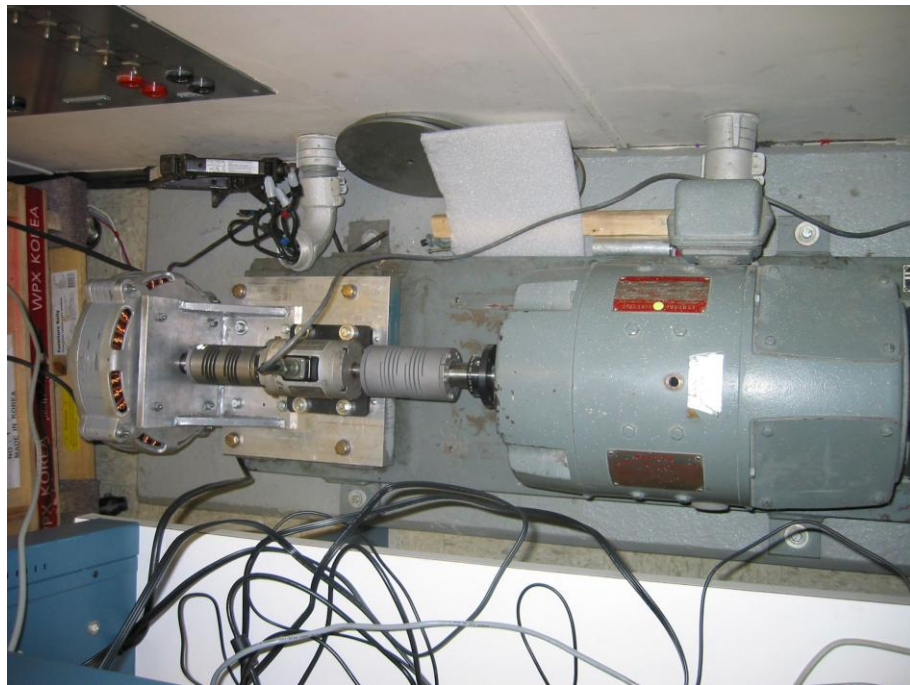
Figure 5-6 PMA-SynRM motor (left) and dynamo load (right) setup
