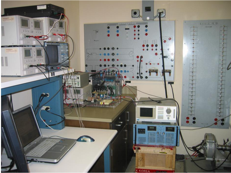
Figure 5-4 Experimental setup of the PMa-SynRM motor drive system
