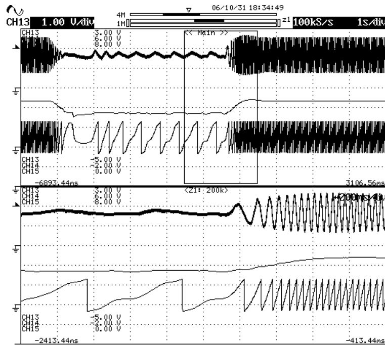
Figure 5-15: (From top to bottom) Phase A current (DSP)-[1V/div], motor speed change-[1V/div] (from 130RPM to 10RPM and back to 130RPM) and estimated position using sliding observer-[1V/div]
